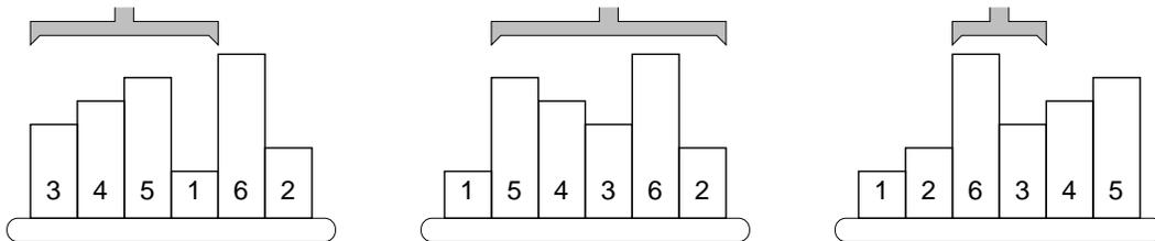
The picture shows a simple example of 6 samples. The smallest one is on the 4th position, therefore, the robot arm reverses the first 4 samples. The second smallest sample is the last one, so the next robot operation will reverse the order of five samples on positions 2–6. The third step will be to reverse the samples 3–4, etc.
